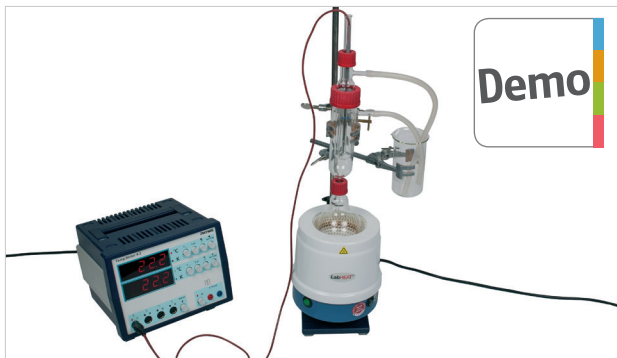
Quantitative experiment: Determination of molar masses via a measurement of the boiling point elevation (ebullioscopy) (P1136000)
